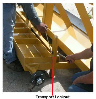
Use Transport Lockout bolt to safely transport scraper.
