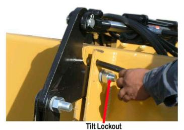
Remove Lockout bolts and nuts (2 each) to use tilt function.
